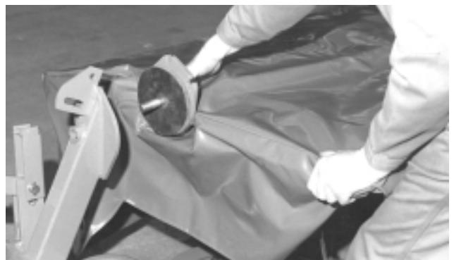
Figure 12 Attaching Curtain Frame To Upright
